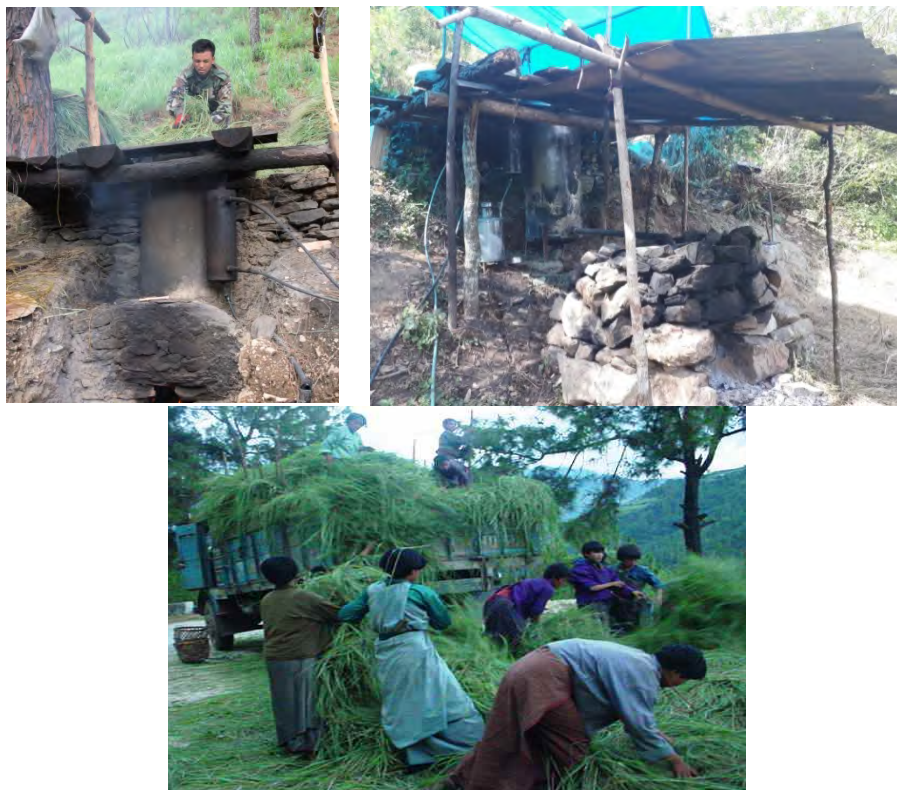
Figure 7: Lemon grass oil extraction using a distillation drum & women loading lemon grass
